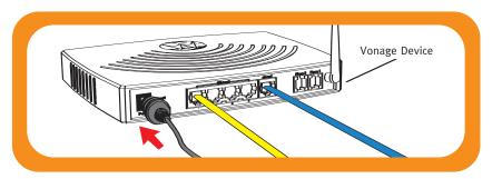
NOTE: Before continuing, the "Power" and "Internet" lights on the front of the Vonage Device should both turn on. Wait until the "Power" light stops blinking and both "Power" and "Phone 1" lights are solid. The "Phone 2" light will be solid if you have a second Vonage line. Otherwise, it will not light. The "Internet" light will flicker whenever there is communication activity.
